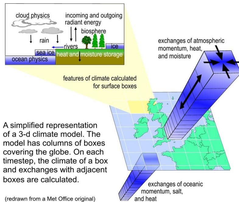
Figure 1: A schematic example of a climate model.
